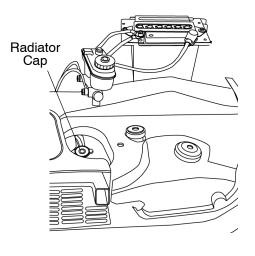
**NOTE:** Use of a non-standard pressure cap will not allow the recovery system to function properly. See your dealer for the correct replacement part.
